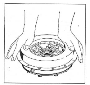
Figure 28. Installing Clutch Cylinders on Bevel Gear Carrier.
